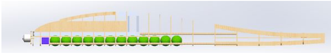
Figure 2: Side View of Loaded Fuselage.
