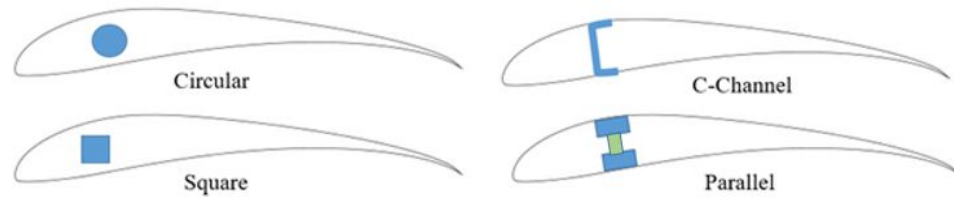
Figure 9.1.1: Proposed Spar Configurations
