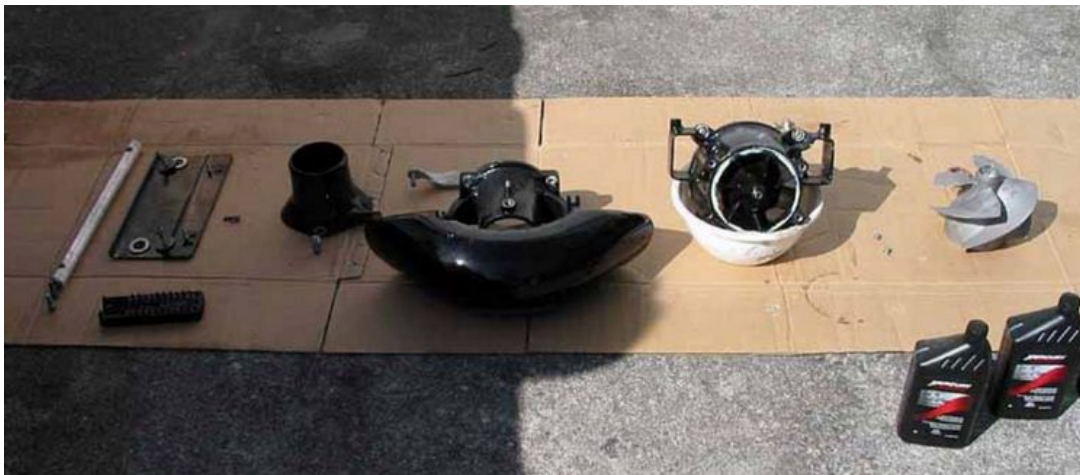
Introduction Figure 1: Parts that must be removed to Access the Impeller and Wear Ring. From Left to Right: Steering Cable, Mounting Bolts/Plate, Flow Nozzle (Rudder), Reversing Gate/Spring, Stator, and the impeller itself, which must be removed to expose the inner surface of the wear ring.
