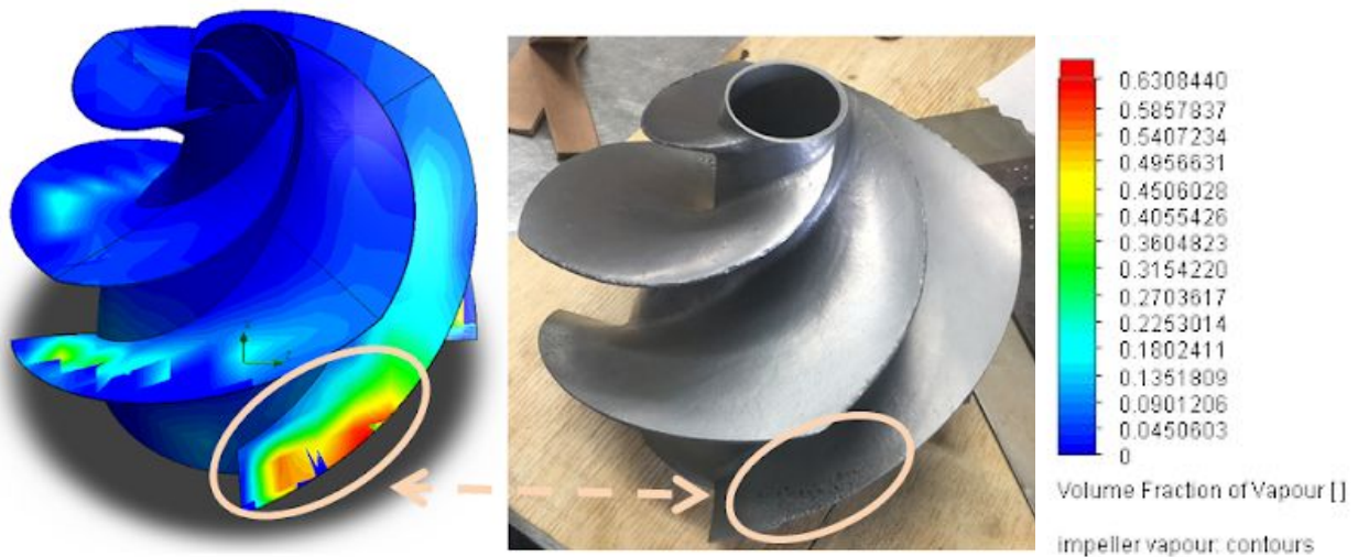
3D fluid vaporization plot (CFD Figure 8)
